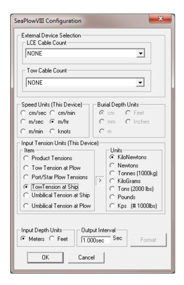
Select the data source for the LCE telephone cable count data and the Tow cable count data from the dropdown lists. Also select the appropriate Input Speed Units and Burial Depth Units as well as each Input Tension Item and its associated Units. Specify whether the Input Depth Units are to be meters or feet and enter an Output Interval.
