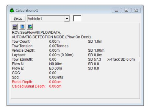
From this window you can monitor some of the input data, as well as the layback calculation. This Calculation window also provides a shortcut to the Configure Plow dialog box by clicking the button.
